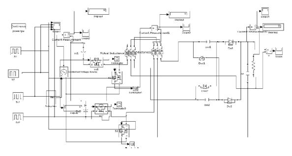
Figure 4. Simulation Model of High Gain Interleaved Boost Converter
