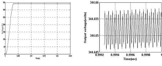
Figure 5. Output Voltage Waveform of High Gain Interleaved Boost Converter
