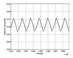
Figure 7. Inductor Current Waveform of High Gain Interleaved Boost Converter
